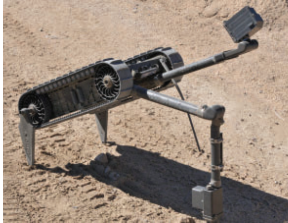
Soldiers use the iRobot 510 PackBot to identify and disarm a simulated improvised explosive device at the Robotics lane at Fort Irwin, Calif. (Army photo.)
