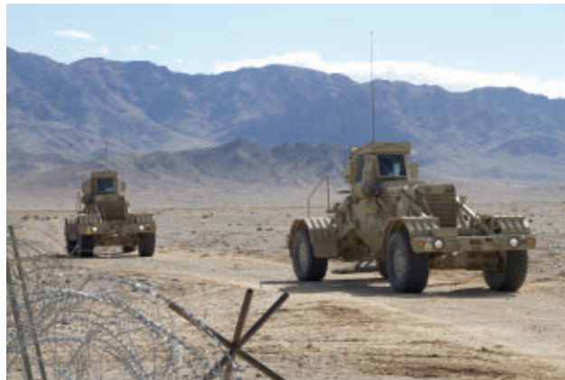
Two U.S. Army Humvee vehicle-mounted mine detection systems use ground-penetrating radar to detect IEDs. (Army photo.)
