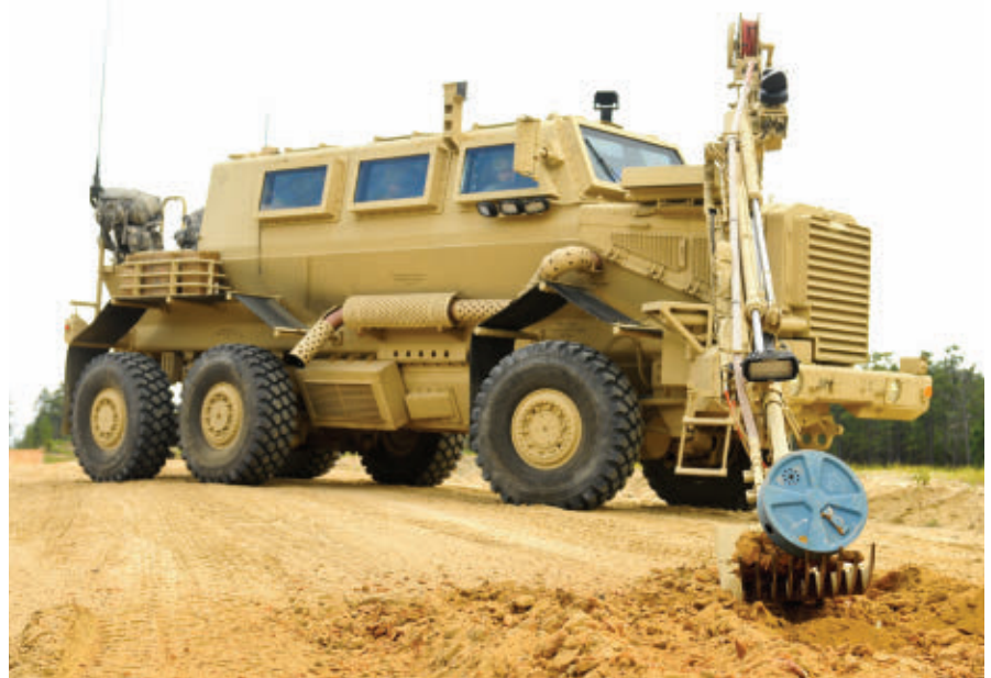
A U.S. Army Buffalo explosive device detection vehicle digs up an improvised explosive device during route clearance operations at McCrady Training Center, Eastover, S.C. (National Guard photo.)
